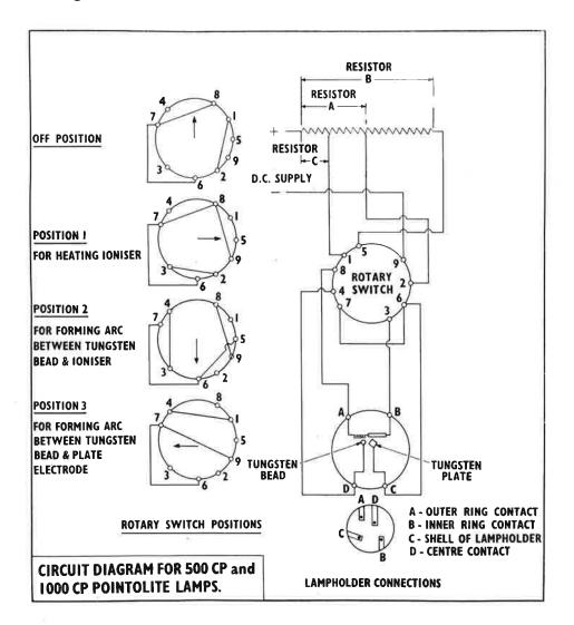
The Rotary Switch shewn in the above diagram must be of the rapid action type, as it is imperative that the change from position 2 to position 3 be made instantaneously.
