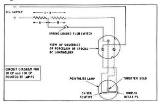
The special three plunger lampholder requires to be wired with three core flexible cable, and it is imperative that the wiring of the lampholder is as shewn above.
